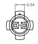
MOUNTING HOLE Ø5.9 CHASSIS THICKNESS 0.6
